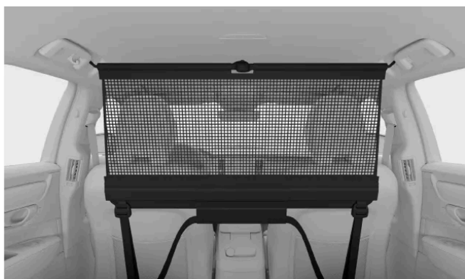
Installing behind second row seats
