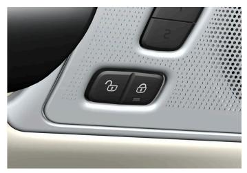
Locking and unlocking button with indicator lamp in the front door.
