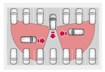
Examples of areas where Cross Traffic Alert can assist the driver to detect obstacles during reversing.
