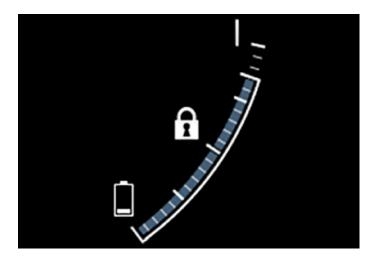
The first symbol in the hybrid battery gauge indicates that the Hold function is activated, and the symbol indicates that the Charge function is activated.
