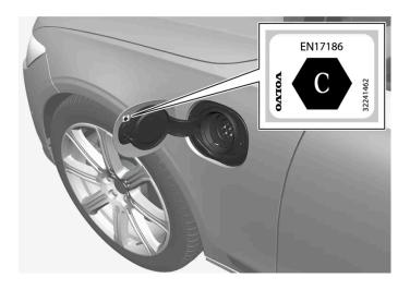
Use charging that is approved for use in the car in accordance with the identifier [1] on the inside of the charging input socket flap.
