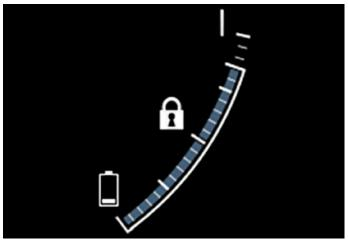
The symbol fi is shown in the hybrid battery gauge when Hold is activated.
