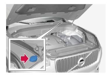
Washer fluid is filled into the reservoir with the blue cap. The reservoir is used for windscreen washer, rear window washer and headlamp washers\*.
