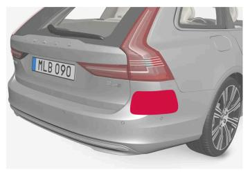
Keep the surface indicated clean – on both the left and right-hand sides of the car<sup>[2]</sup>.
