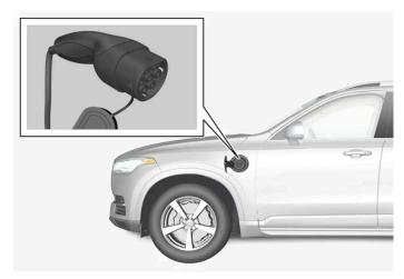
Charging cable handle and charging input socket.
