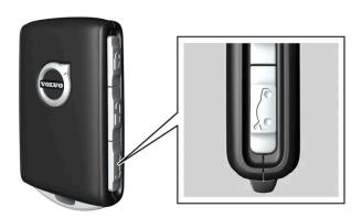
Unlocking the tailgate by pressing a button:
