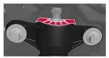
Turn the adjuster knob clockwise and anticlockwise respectively to change adjustment position.
