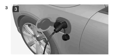
Position the charging handle's protective cover so that it does not touch the car.
