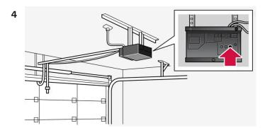
Locate programming button<sup>[2]</sup> on the receiver for the garage door or similar. It is normally located close to the antenna's bracket on the receiver.
