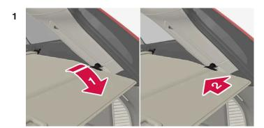
Grip the handle and pull the cargo cover out to the end position.
