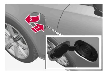
1 Press in the rear section of the cover and release.
