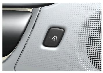
Lock button with indicator lamp in the rear door.
