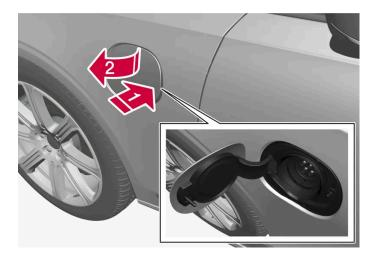
Press in the rear section of the cover and release.
