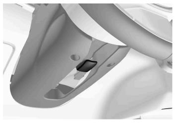
Lever for steering wheel adjustment.
