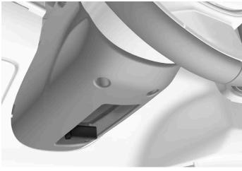
Lever for steering wheel adjustment.
