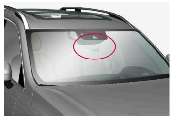
Location of front camera and radar unit
