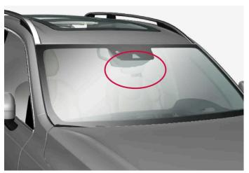
Location of front camera and radar unit
