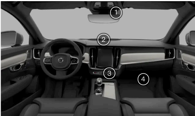
The interior climate sensors
