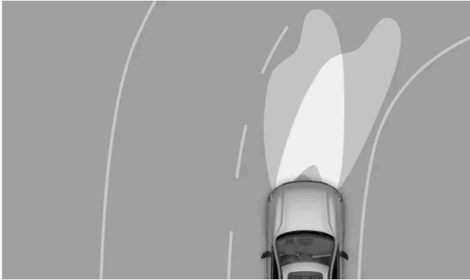
The active bending lights
