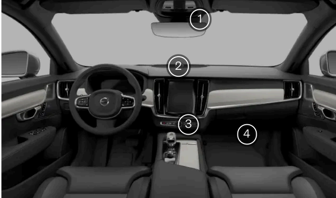
The interior climate sensors
