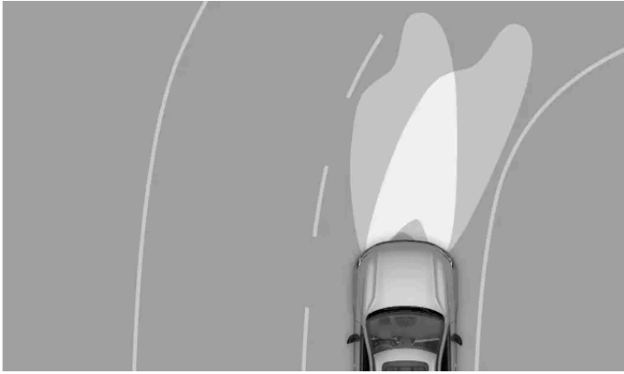
The active bending lights
