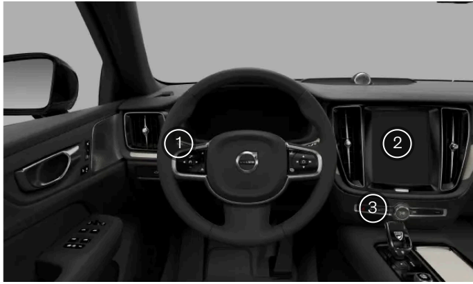
Exterior lights controls locations
