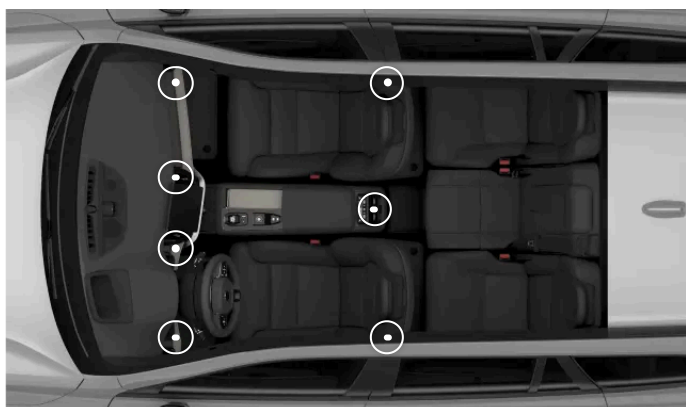
The locations of the adjustable air vents
