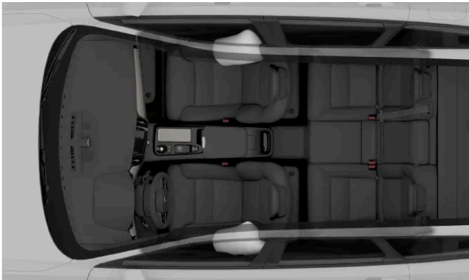
Side collision airbags for the front occupants.
