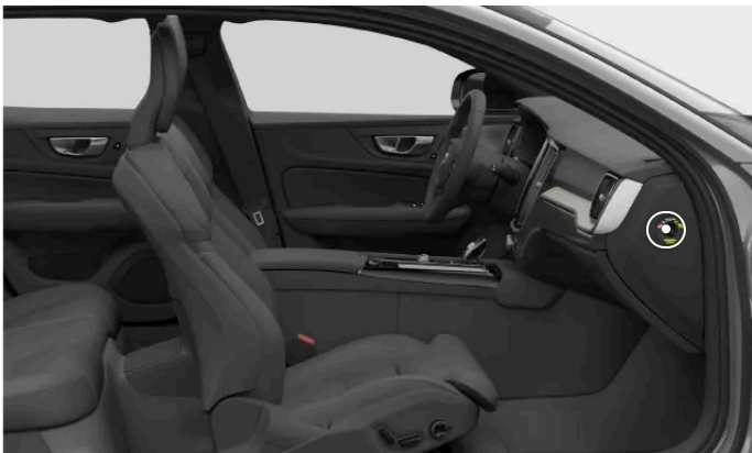
Location of the passenger airbag switch
