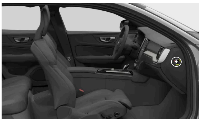
Location of the passenger airbag switch
