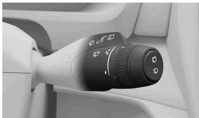
Right-hand steering wheel stalk
