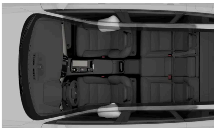
Side collision airbags for the front occupants.
