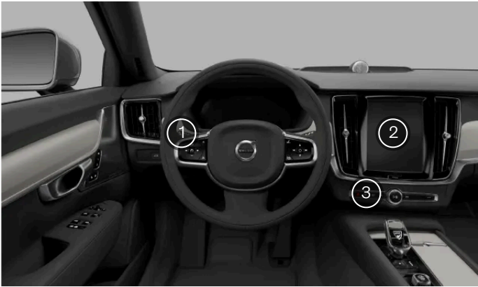
Exterior lights controls locations
