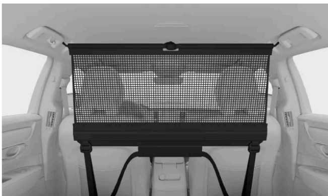
Installing behind second row seats
