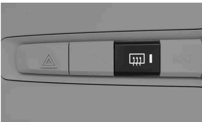
Rear defroster button on the button panel below the centre display
