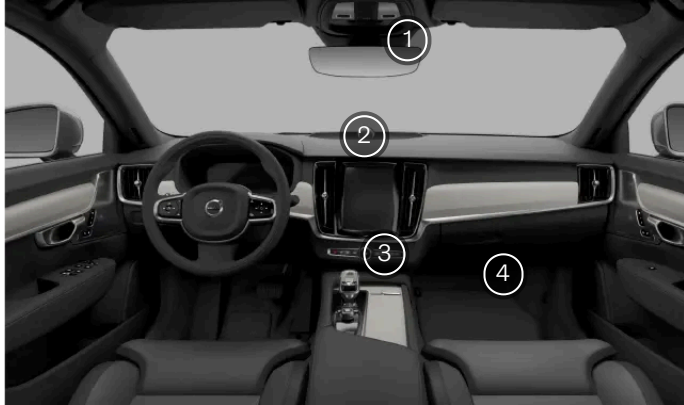
The interior climate sensors
