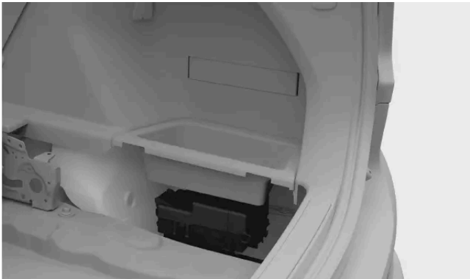
Fuse box location
