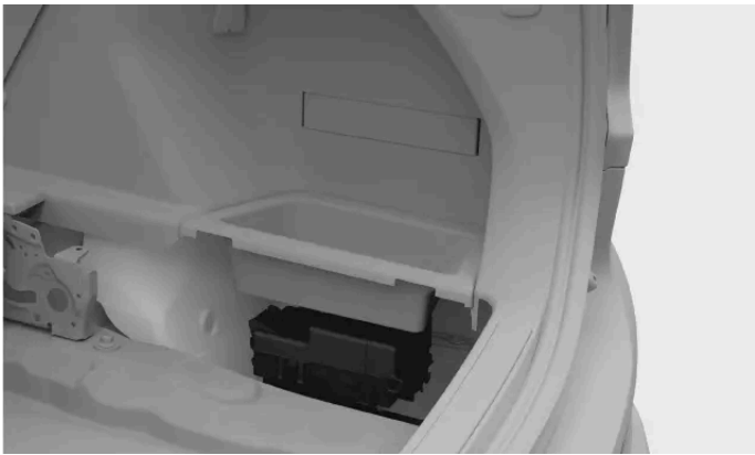
Fuse box location
