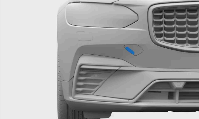
Front towing eye fastening cover
