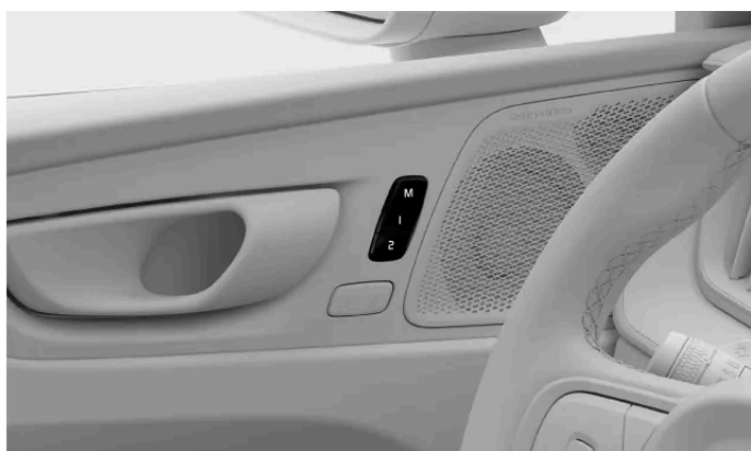
Location of the preset seat adjustment buttons
