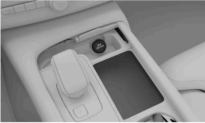
The 12 V socket in the tunnel console
