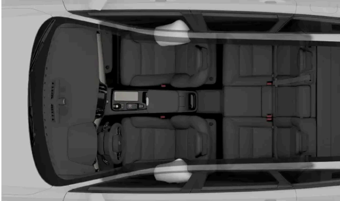
Side collision airbags for the front occupants.
