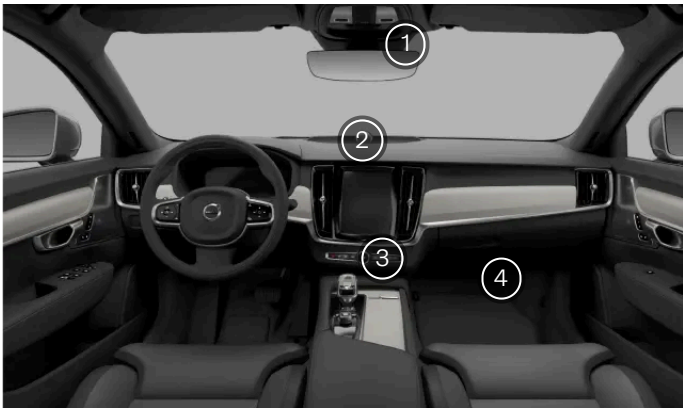
The interior climate sensors
