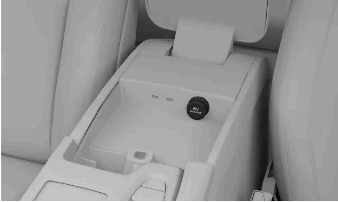
The 12 V electrical socket in the tunnel console
