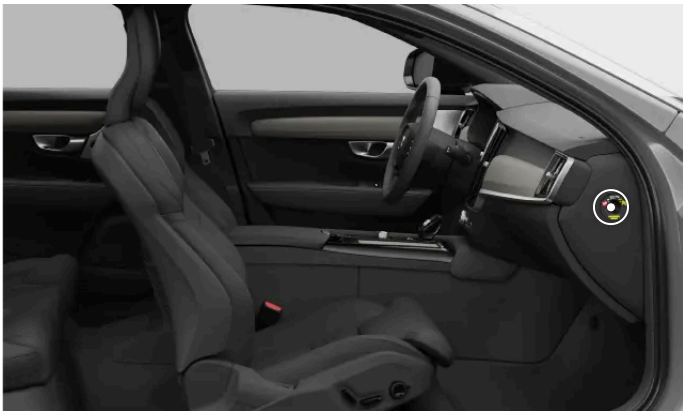
Location of the passenger airbag switch
