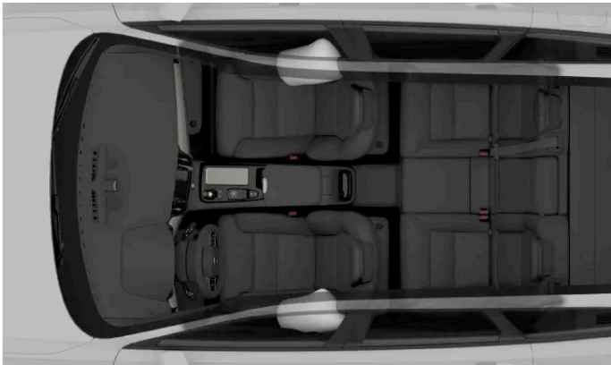
Side collision airbags for the front occupants.
