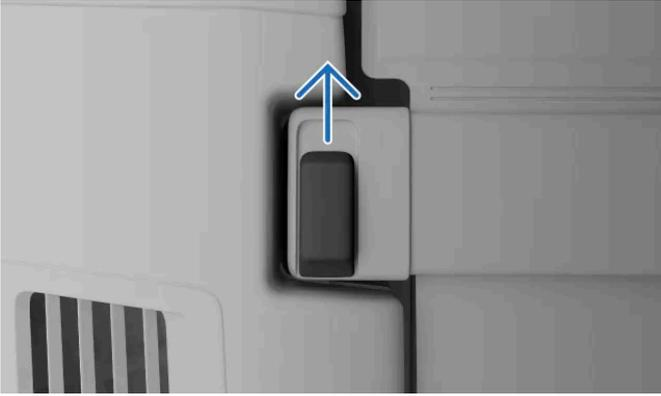
There are lock buttons at the ends of the load cover. Push the button on one side forwards and hold it in place while lifting the end of the load cover. Do this for the other end of the load cover as well.
