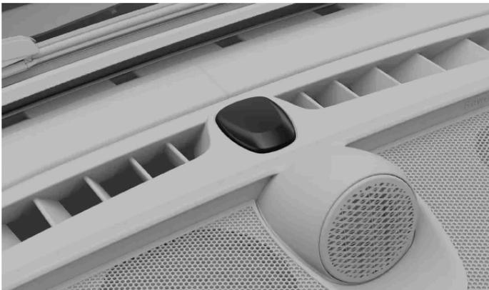
The alarm indicator is a light located in the centre of the dashboard, just in front of the windscreen. The indicator confirms when the alarm is enabled with a flashing red light.
