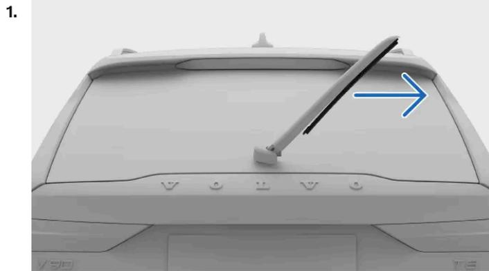
Grasp the centre of the wiper arm and lift it up and away from the rear windscreen. You may feel some resistance halfway – this is the lock position. You need to pull the wiper arm past the lock position so that it doesn't fall back onto the windscreen.
