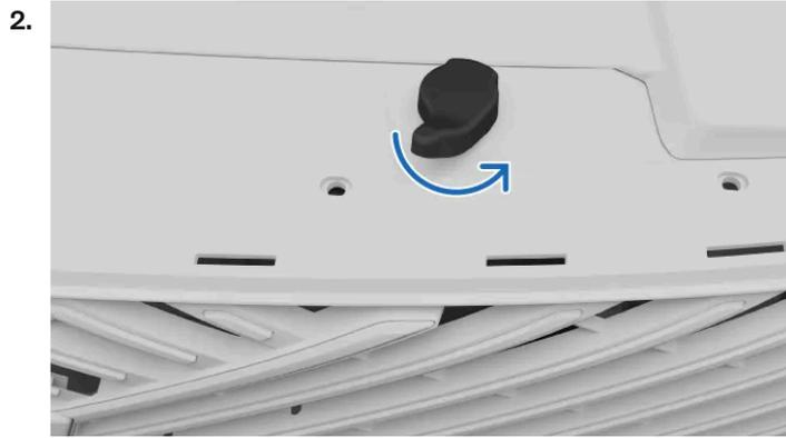
Locate the second lever below the front edge of the bonnet and rotate it anticlockwise.
