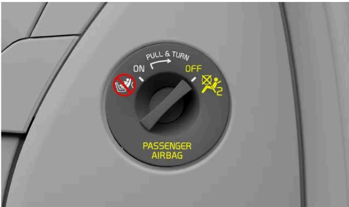
Airbags disabled. Always use this position when a rearward-facing child restraint is installed in the front passenger seat.
