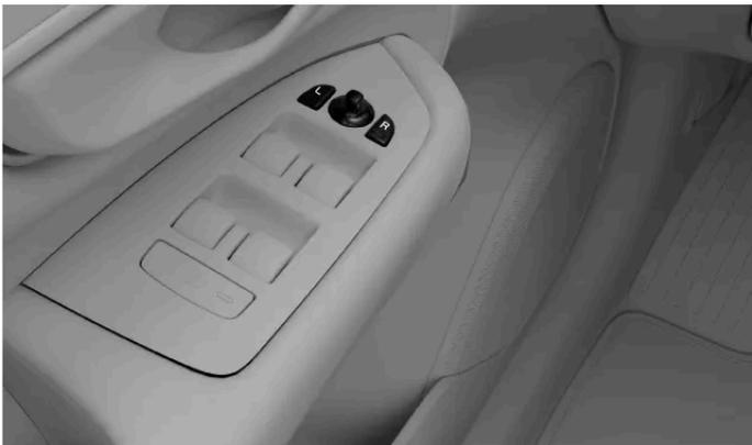
Controls for adjusting the wing mirrors
