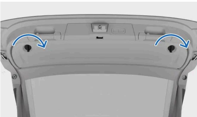
The warning triangle is located on the inside of the boot hatch. Open the compartment by turning the handles so that they are vertical and then pulling it.
