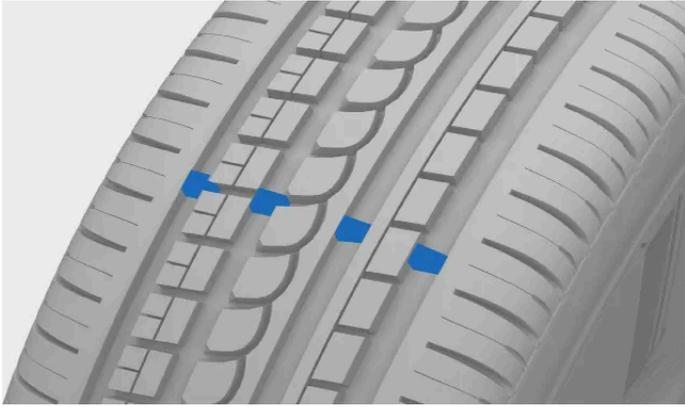
The narrow grooves that run lengthways across the tyre's tread pattern are tread wear indicators. On the side of the tyre are the letters TWI <sup>[1]</sup>.
