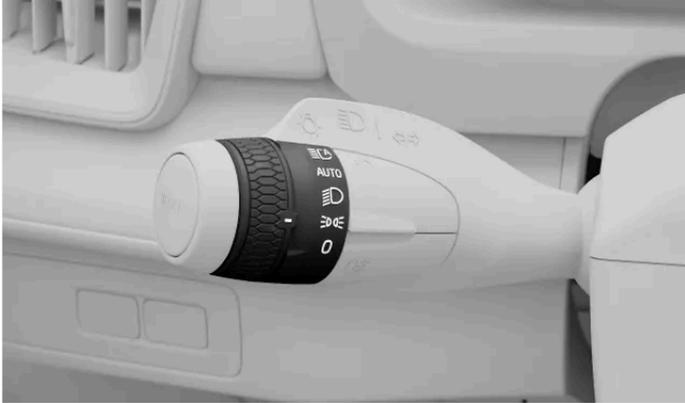
The position lights symbol on the rotating ring on the left-hand stalk
