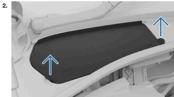
Open the panel hatch in the upper-left corner of the engine compartment to access the coolant container.
