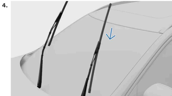
Make sure that the blade for the driver side is longer than the blade for the passenger side. Slide the wiper blade onto the wiper arm. Ensure that the pin on the wiper arm goes into the hole on the wiper blade. Push the blade into the wiper arm until you hear a click sound.
