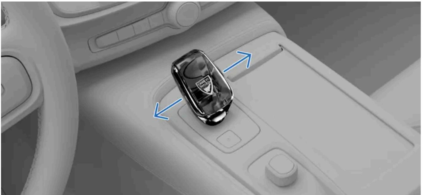
After selecting gear B, you can manually shift gears by moving the gear selector to the left or right.
