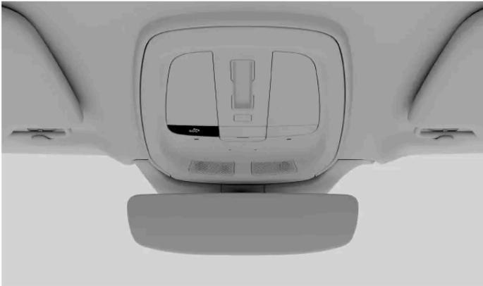
The SOS button is located in the ceiling, on the left side of the overhead console.
