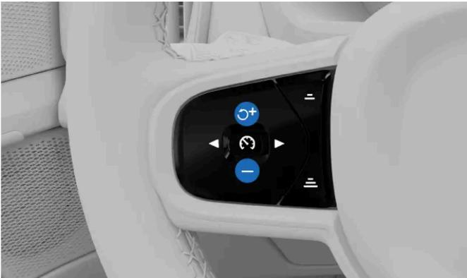
Adjust the target speed using the buttons on the steering wheel.
