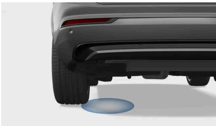
The sensor picks up movement under the rear bumper. Any detected movements unlock the boot.
