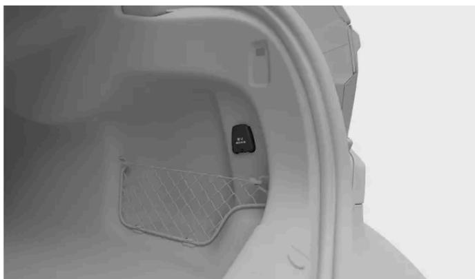
The 12 V electrical socket on the right-hand side in the boot
