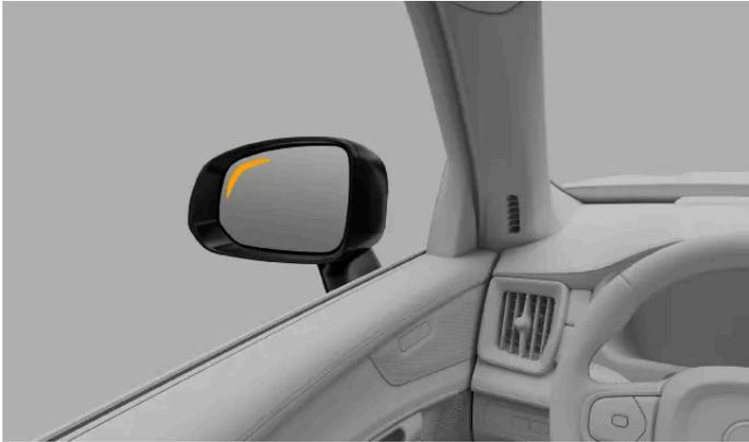
When a vehicle is detected in or approaching your blind spot, a light appears in the wing mirror.
