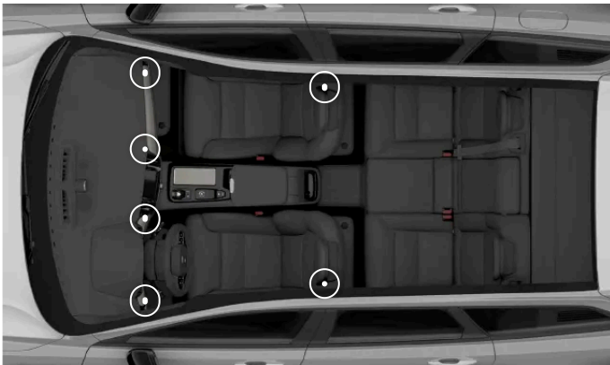
The locations of the adjustable air vents
