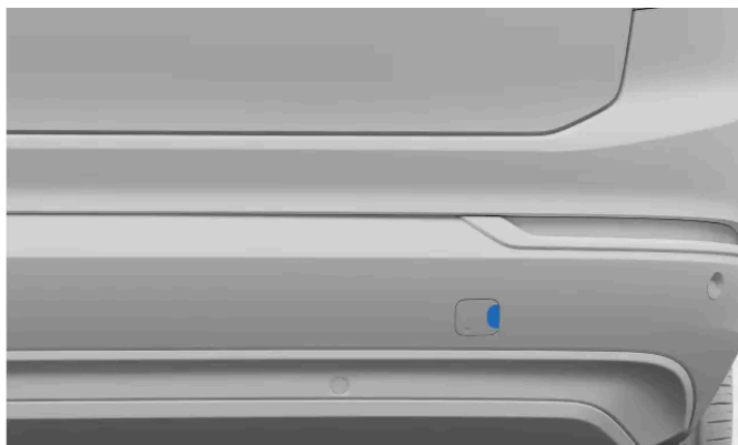
Rear towing eye fastening cover
