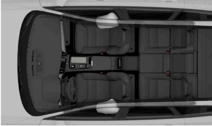
Side collision airbags for the front occupants.
