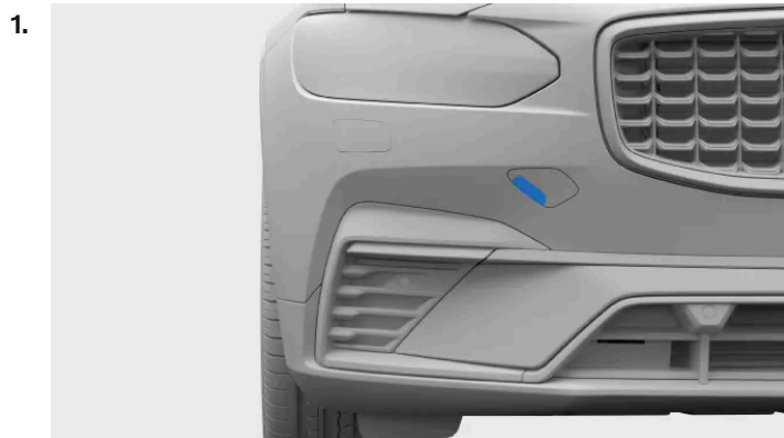
Front towing eye fastening cover
