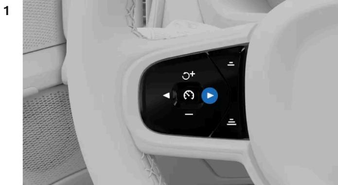
1 Press the switch button **▶** on the steering wheel.
