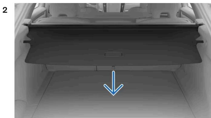
Pull the load cover screen by the handle over the boot's side panels.
