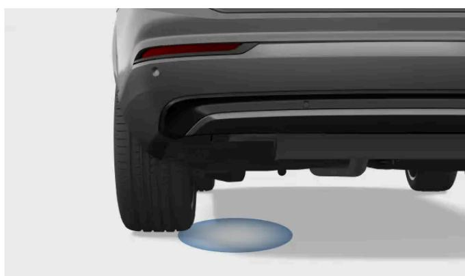
The sensor picks up movement under the rear bumper. Any detected movements unlock the boot.
