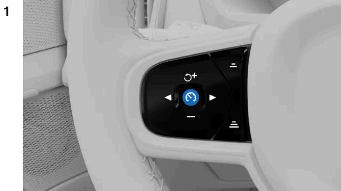
When it's safe to do so, press the Pilot Assist button
