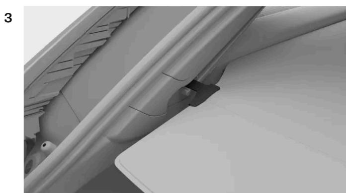
Guide the ends of the load cover into the locked position in the grooves.
