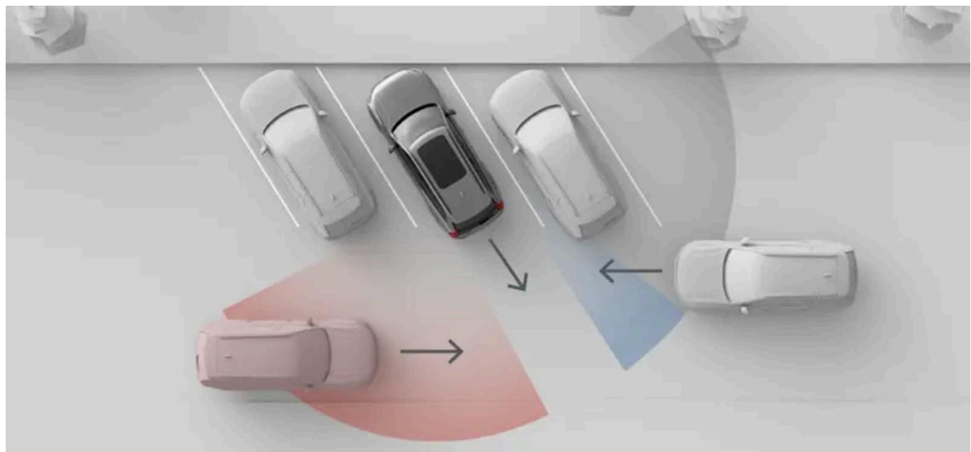
The situation shown in this image illustrates how surrounding objects, such as parked cars can limit the car's ability to detect other vehicles and traffic situations. In a situation without obstacles, the effective detection zones are the same on both sides.
