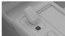
When P is selected, the gearbox is mechanically blocked to avoid accidental gear shifts.
