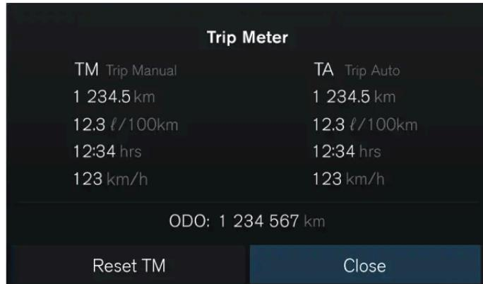
Your car has a trip meter and an odometer. The trip meter can show information on the car's driving distance and time, as well as your average fuel consumption and driving speed.
