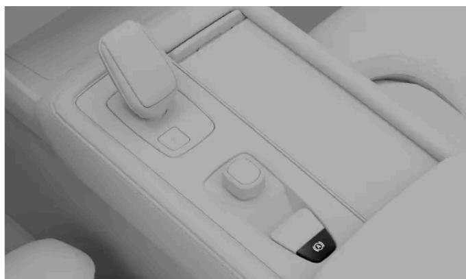
**1** Press the auto hold button in the tunnel console.
