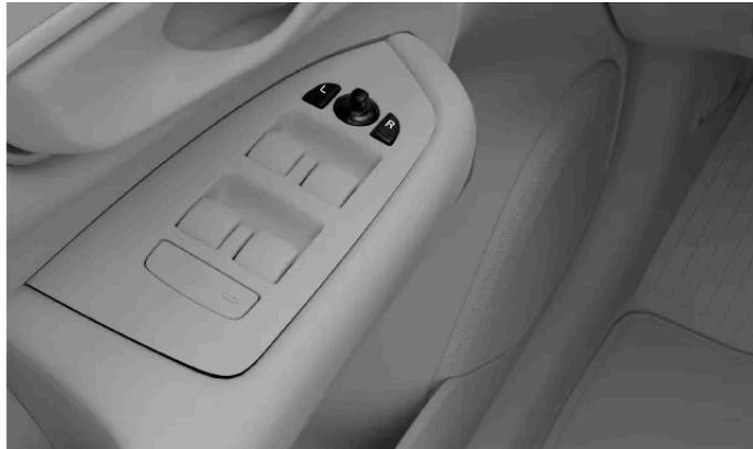
Controls for adjusting the wing mirrors
