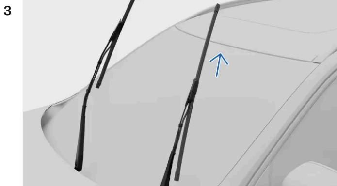
Press the button on the wiper arm and remove the wiper blade by pulling it upwards.
