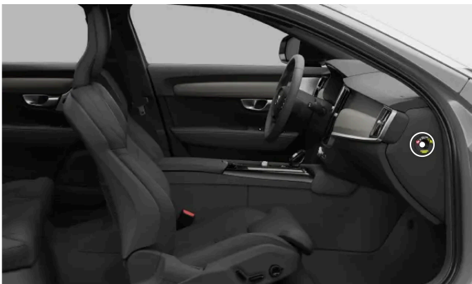
Location of the passenger airbag switch
