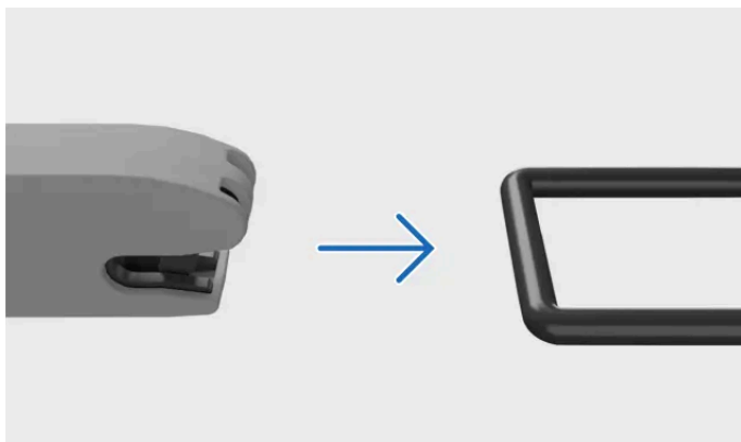
Attaching to ISOFIX anchorage point
