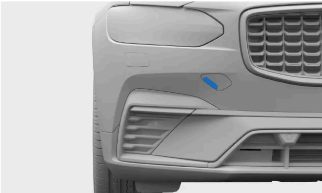
Front towing eye fastening cover
