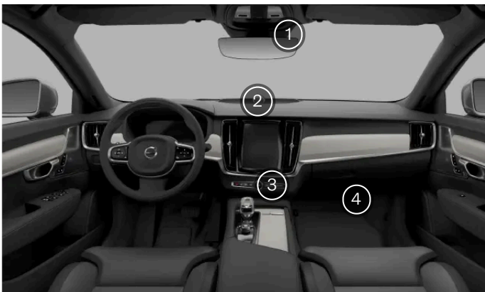
The interior climate sensors
