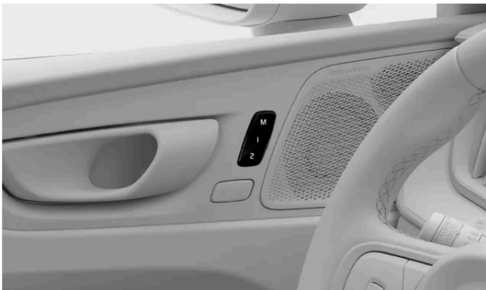
Location of the preset seat adjustment buttons
