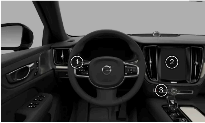
Exterior lights controls locations
