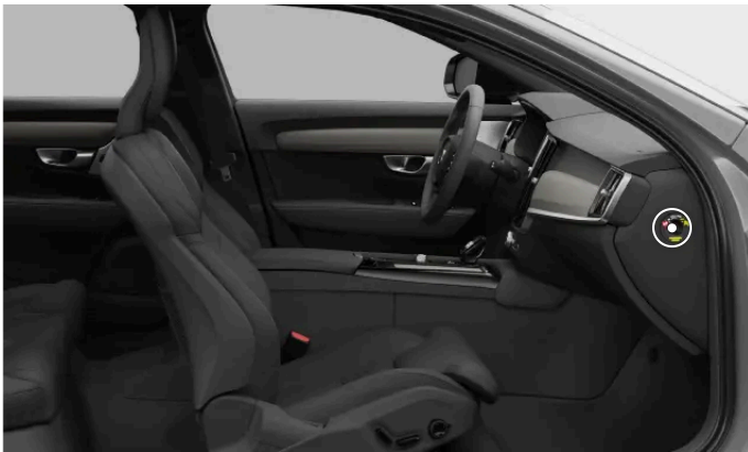
Location of the passenger airbag switch
