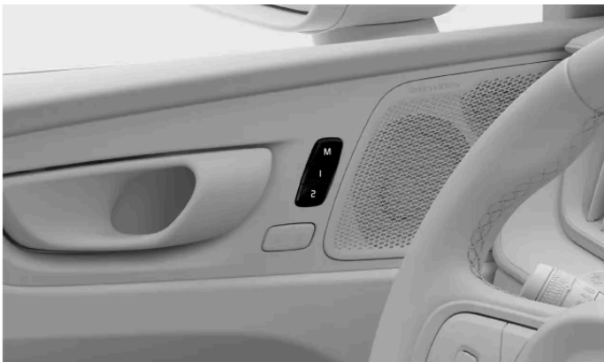
Location of the preset seat adjustment buttons
