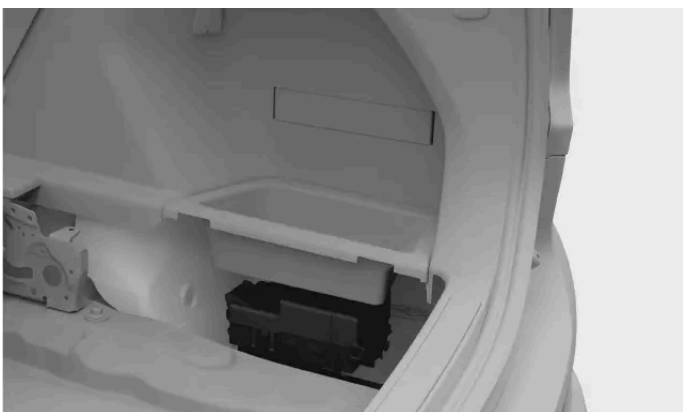
Fuse box location
