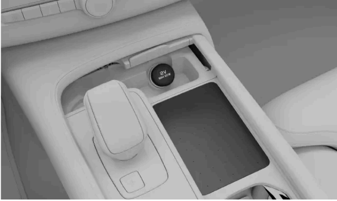
The 12 V socket in the tunnel console
