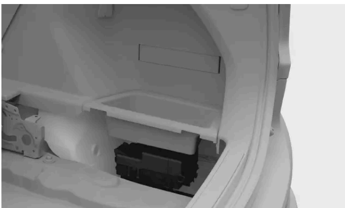
Fuse box location
