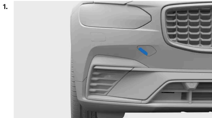
Front towing eye fastening cover
