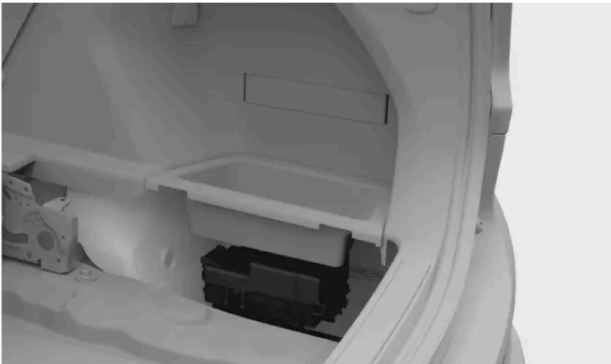
Fuse box location
