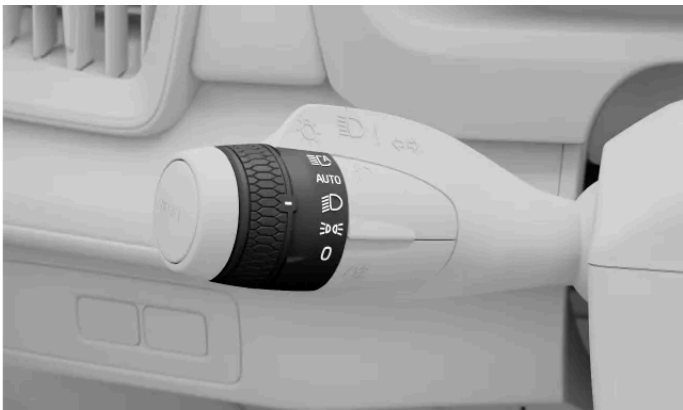
The passing beam symbol on the rotating ring on the left-hand stalk
