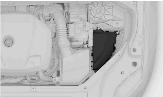
Fuse box location
