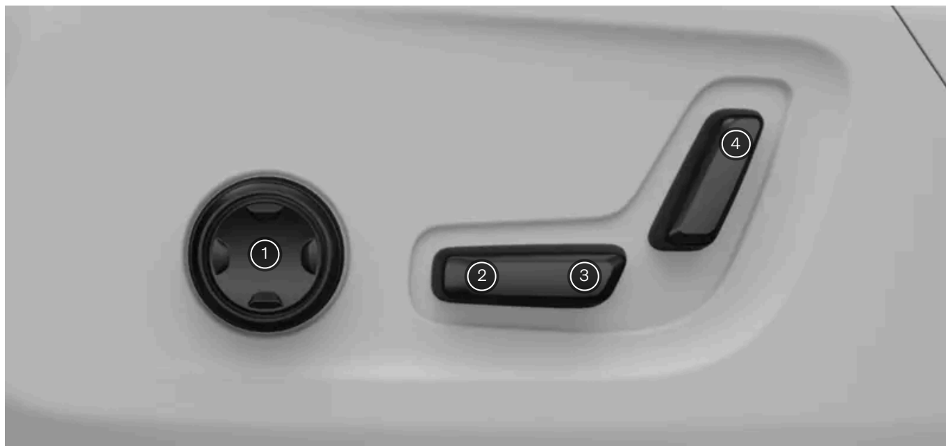
Controls on the side of the seat
