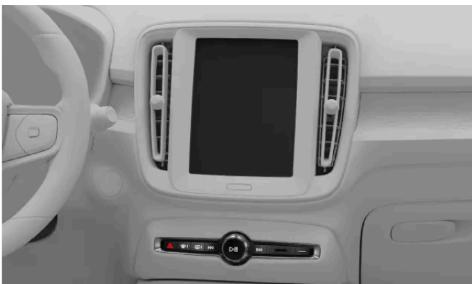
Centre display and defroster buttons on the button panel below the centre display
