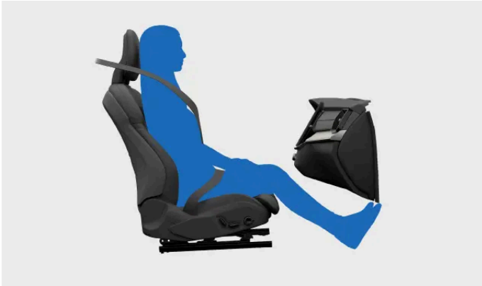
A correctly seated occupant. Do not adopt other postures when the car is moving.
