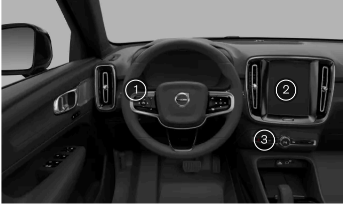
Exterior lights controls locations
