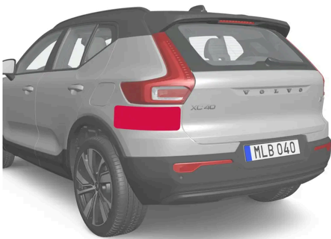
Location of rear radar units
