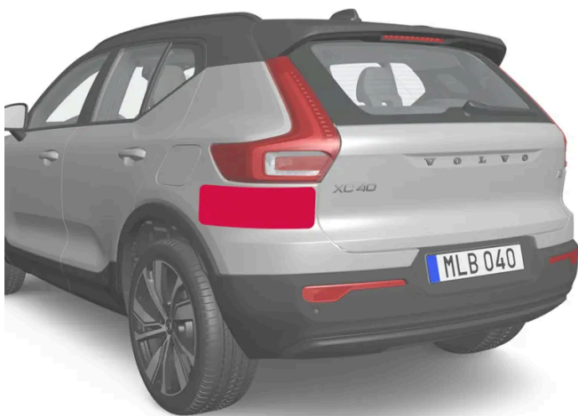
Location of rear radar units
