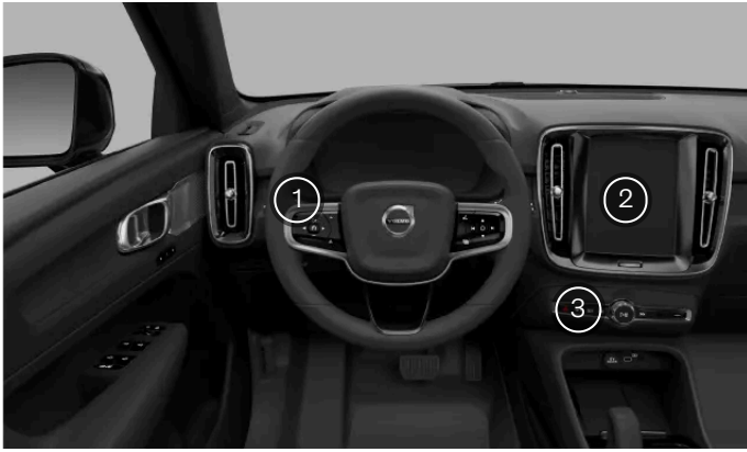
Exterior lights controls locations
