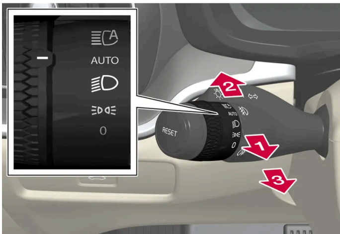
Steering wheel stalk switch with rotating ring.
