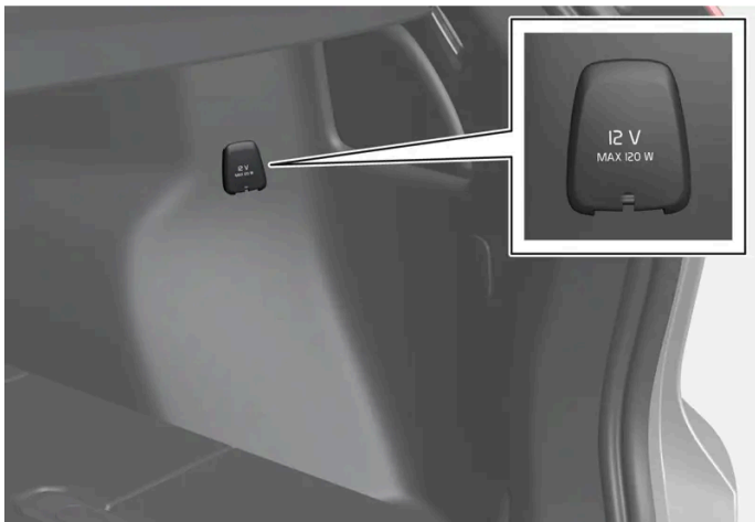
12 V electrical socket in cargo area*, [1]
