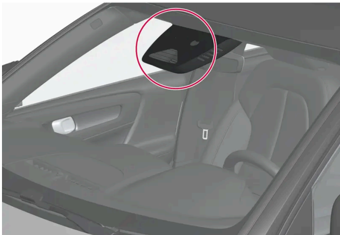
Location of the camera unit
