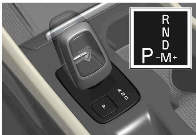
Overview of gear lever and shift pattern in the driver display.
