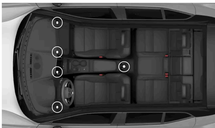
The locations of the adjustable air vents
