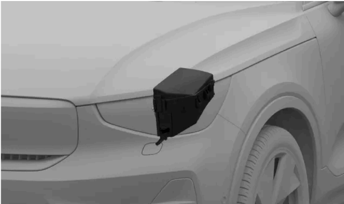
Fuse box location
