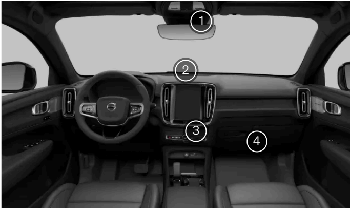
The interior climate sensors
