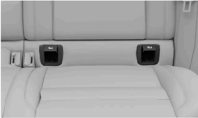
Locations of ISOFIX anchorage points for the outer rear seats
