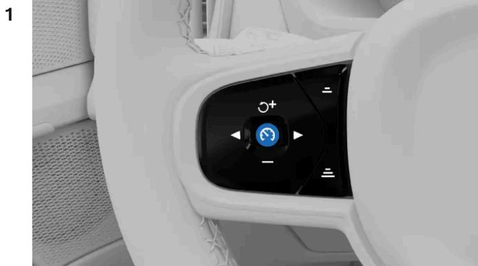
When it's safe to do so, press the Pilot Assist button
