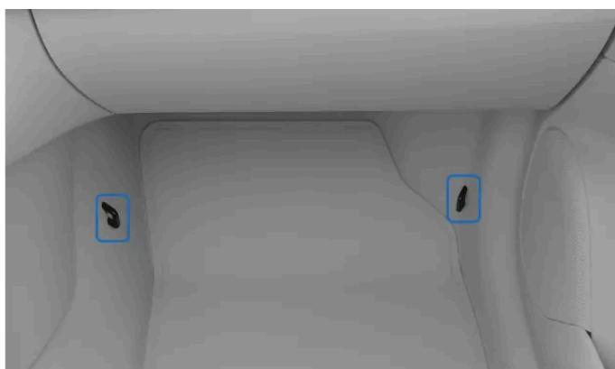
The lower tether anchorage points for the front passenger seat are located on the sides of the seat's footwell.
