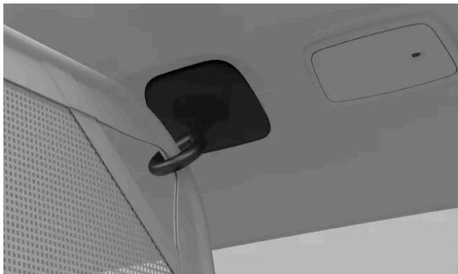
6 Fasten the lower corners of the net to the load-retaining eyelets behind the seats.
