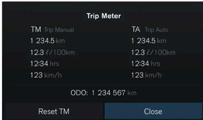
Your car has a trip meter and an odometer. The trip meter can show information on the car's driving distance and time, as well as your average fuel consumption and driving speed.
