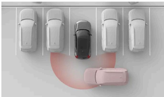
Your car can detect a car crossing behind you, for example when reversing out of a parking spot. This allows it to warn you so that you can slow down or brake.
