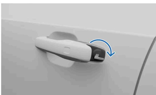
5 Turn the key back 45 degrees anticlockwise back to its starting position and remove it.
