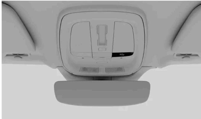
The assist button is located in the ceiling, on the right side of the overhead console.
