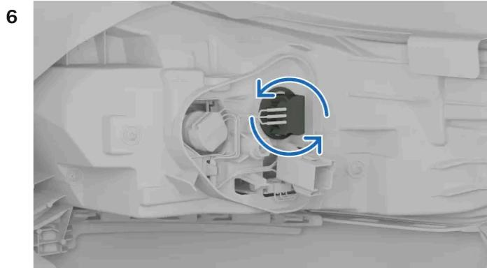
Turn the grey bulb holder anticlockwise and pull it out.
