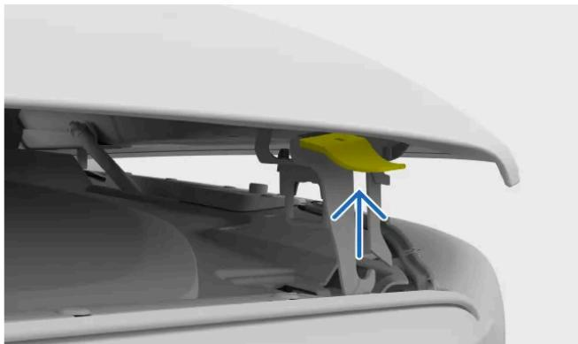
Locate the second lever on the underside of the bonnet and push it upwards.
