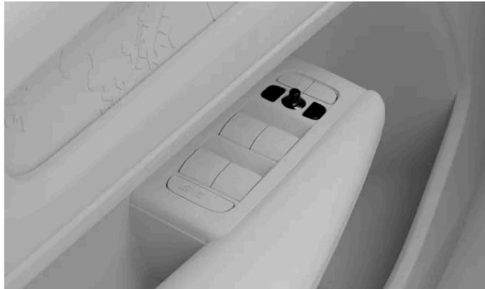
Controls for adjusting the wing mirrors
