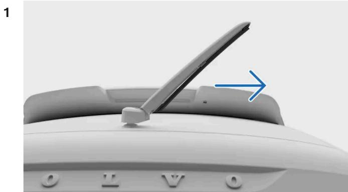
Grasp the centre of the wiper arm and lift it up and away from the rear windscreens. You may feel some resistance halfway – this is the lock position. You need to pull the wiper arm past the lock position so that it doesn't fall back onto the windscreens.
