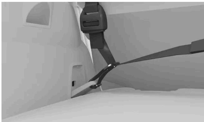
7 Fasten the lower corners of the net to the load-retaining eyelets behind the seats.
