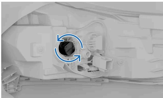
Turn the black bulb holder anticlockwise and pull it out.
