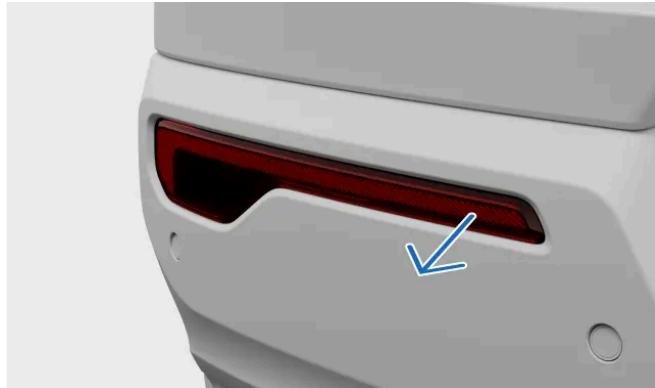
Insert a screwdriver behind the fog light's narrower short side and pry it out.
