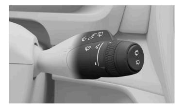
You control the wipers and washers using the right-hand steering wheel stalk.
