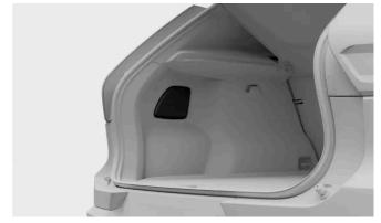
Press the top edge of the panel cover to make it pivot and remove it.
