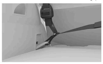
**7** Fasten the lower corners of the net to the load-retaining eyelets behind the seats.
