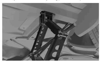
8 Raise the car to an appropriate height. Do not raise it higher than what's necessary for the work you're doing.
