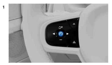
When it's safe to do so, press the Pilot Assist button (5) on the steering wheel.
