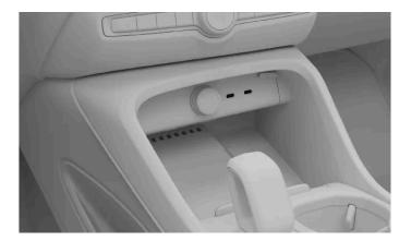
There are also two USB ports in the rear part of the tunnel console.
