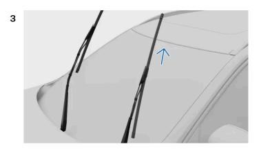
Press the button on the wiper arm and remove the wiper blade by pulling it upwards.
