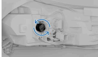
Turn the black bulb holder anticlockwise and pull it out.
