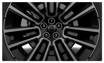
Tighten the wheel fasteners crosswise.
