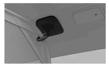
Fasten the lower corners of the net to the load-retaining eyelets behind the seats.
