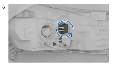
Turn the grey bulb holder anticlockwise and pull it out.
