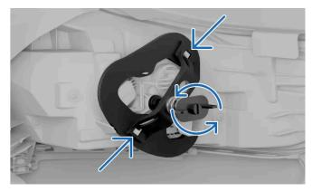
Unscrew the spring screw by turning anticlockwise. Leave the screw in the support bridge so that you can find it when you need it again.
