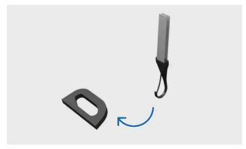
Fastening tether to lower tether anchorage point
