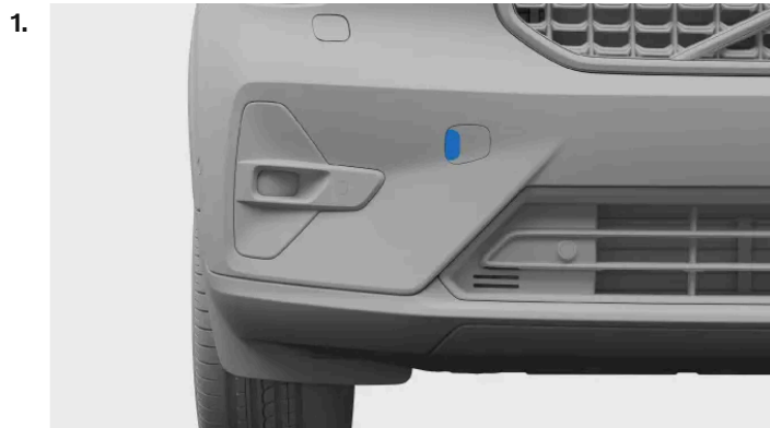
Front towing eye fastening cover
