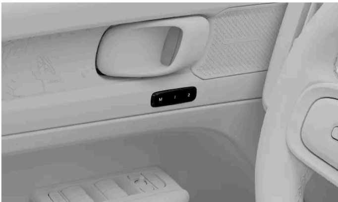
Location of the preset seat adjustment buttons
