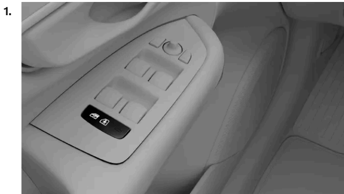
Location of the child lock button in the door panel
