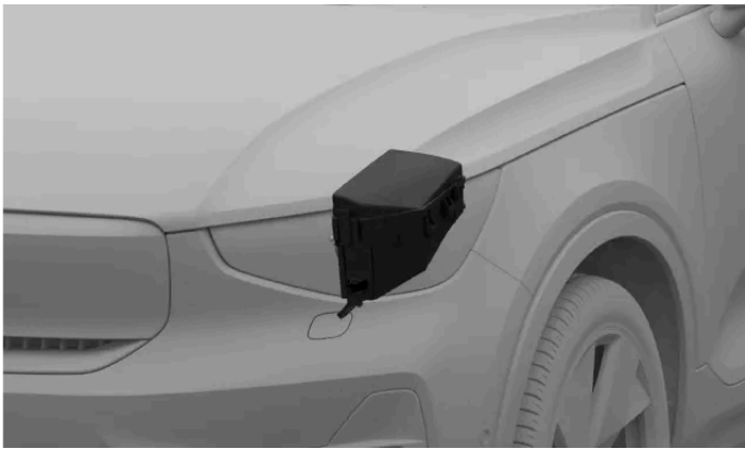
Fuse box location
