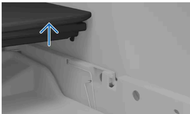
Cargo hatch released.
