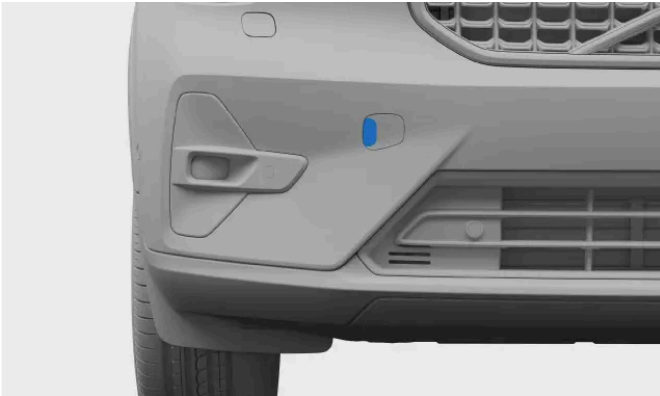
Front towing eye fastening cover
