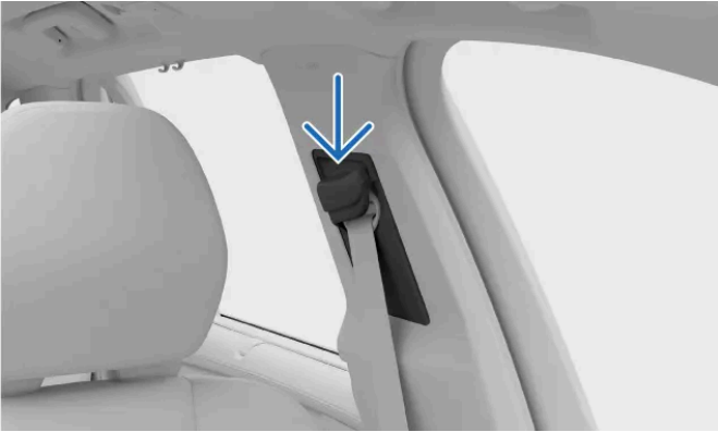
Seatbelt upper anchor point
