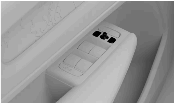
Controls for adjusting the wing mirrors
