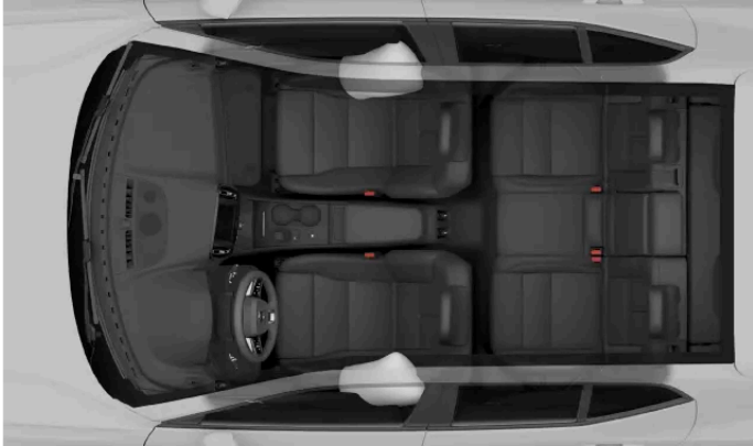
Side collision airbags for the front occupants.
