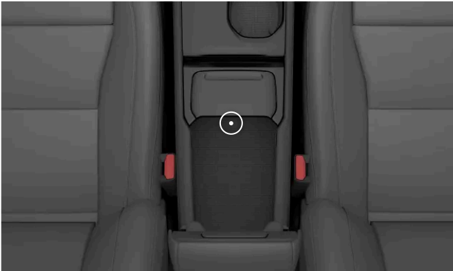
Location of the backup reader inside the tunnel console's storage compartment
