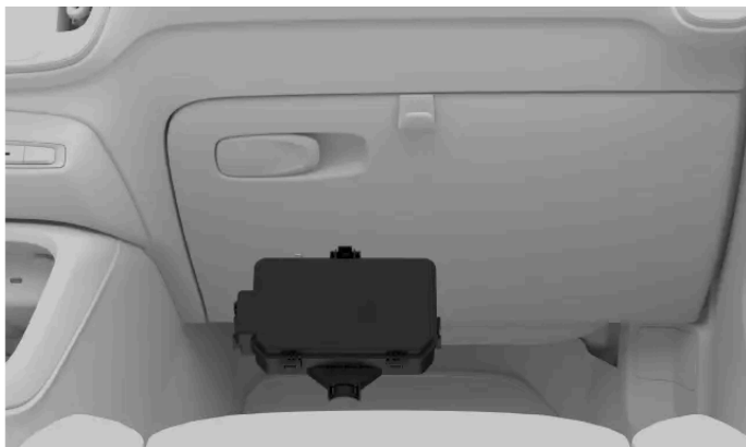
Fuse box location
