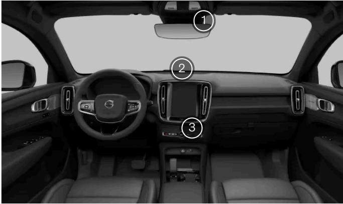
The interior climate sensors
