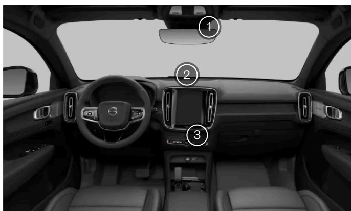
The interior climate sensors
